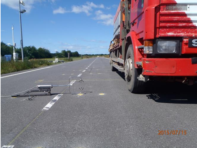
Sensor position: 0.2 m from the road surface, 3.25 m from the center
