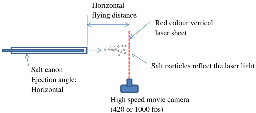
Figure 10: Salt particle reflects red laser light, which enables to capture the moment when the salt-swarm-front passing through the laser sheet on the high speed movie. air transportation. So, the landing velocity of about  $6 \text{ m s}^{-1}$  is lesser than what found during real salt spreading.
