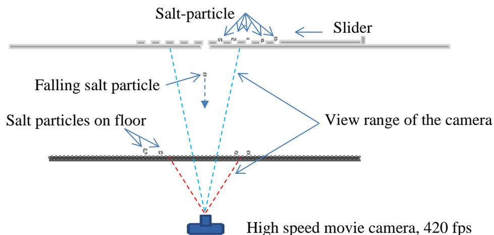
Figure 7: Sketch of the free-fall test
