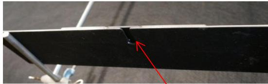
Back side of the guide-plate (The slot enables to observe the salt particles arriving to the edge of the opening)
