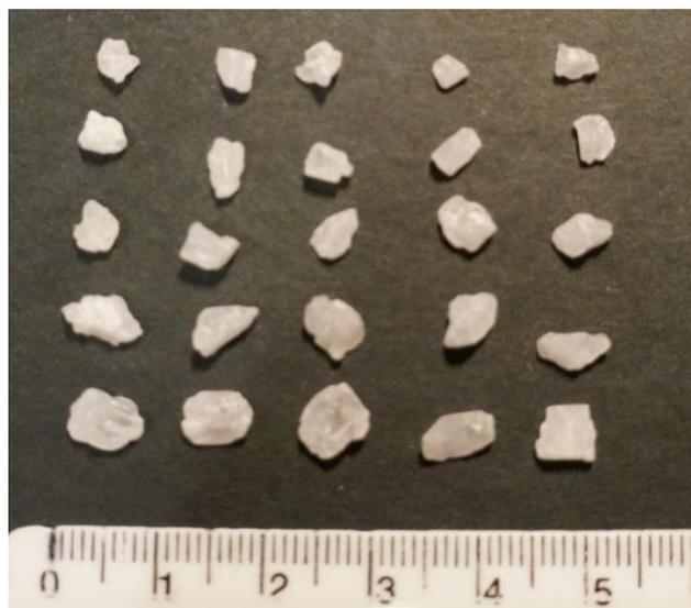
Figure 2: Size and shape variation of rock salt particles.
