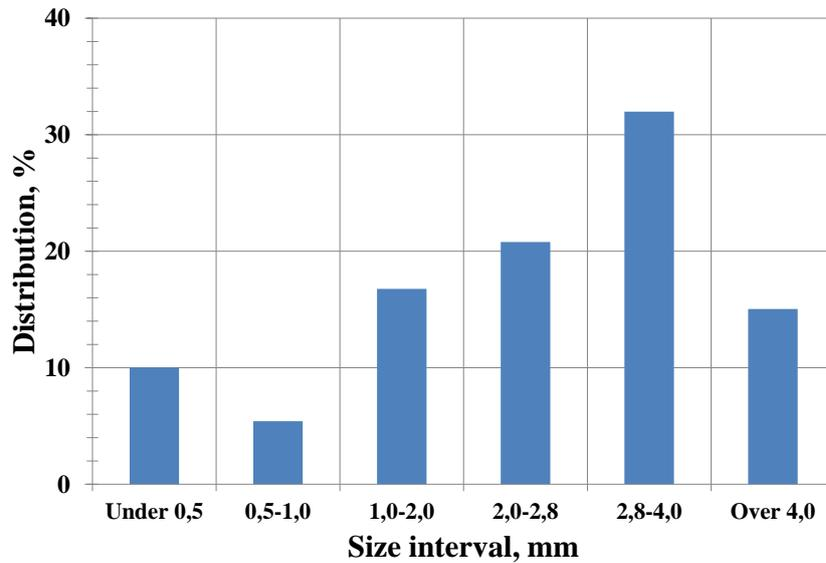
Figure 3: Mass distribution for six size intervals for the sample of rock salt.
