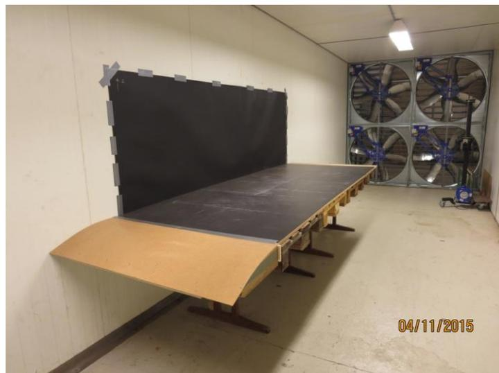
*Figure 1. Wind tunnel with wind table.*
