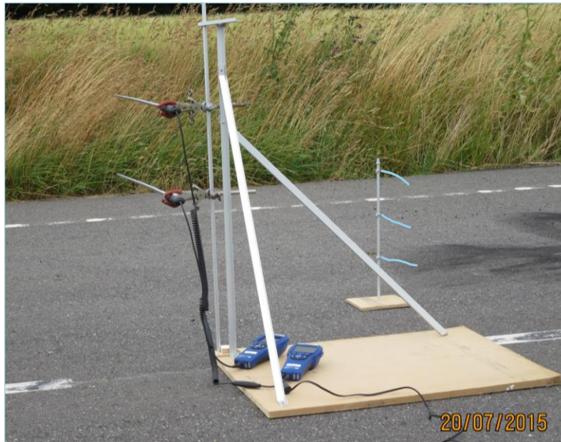
Figure 6. The small test rig carried the two anemometers close to the test road.
