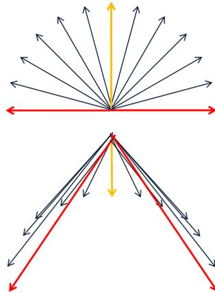
Figure 6. Salt particle velocity relative to the road from a truck at stand still (top) and from a truck moving (bottom).
