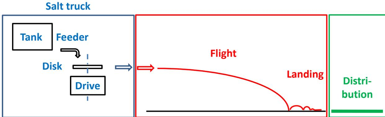
Figure 1. Vertical view of the 3S model for salt spreading from the tank to the road.
