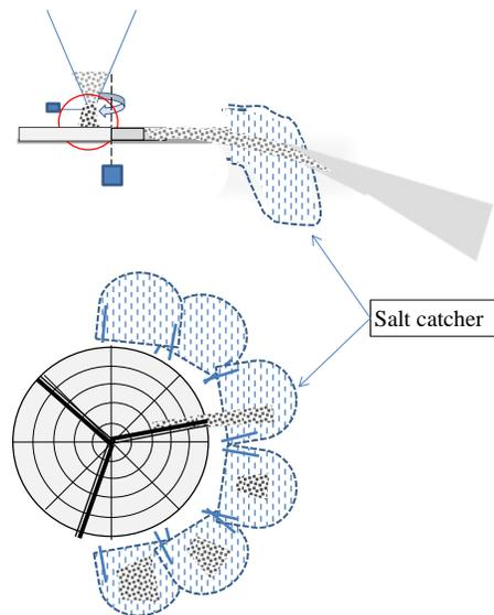
Figure 6. Idea of test set-up to determine spread evenness.
