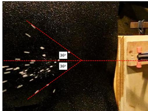
Figure 9. Horizontal view of dry salt particles bouncing of a surface
