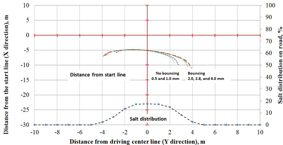
Figure 11. Distance from the start line to the end of first bounce (top) and simulated salt distribution (bottom).
