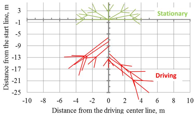
Figure 10. Simulation of symmetric spreading including bouncing of 4 mm rock salt.
