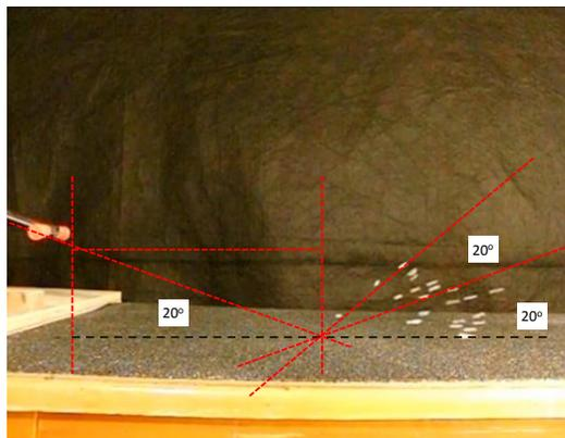
Figure 8. Side view of dry salt particles bouncing off a horizontal surface
