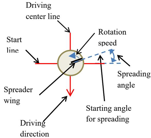
Figure 4. Definition of salt mass cast in different directions
